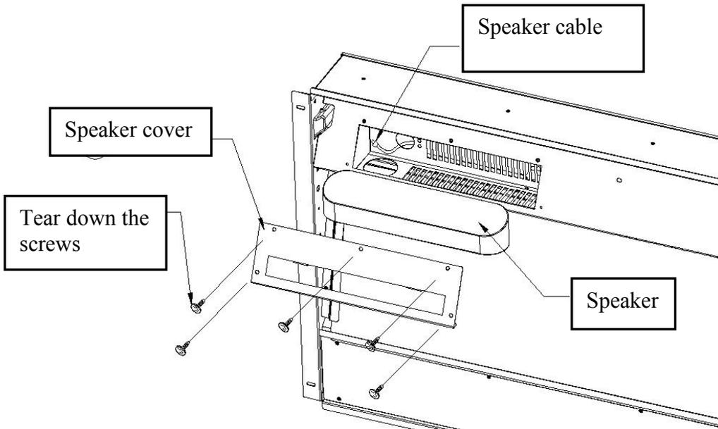
Tear down the screws on the speaker cover, Take out the speaker, Plug out the speaker cable, and cover the speaker
