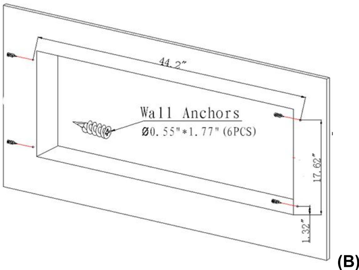
**STEP A.** Selection a dry wall to open a hole for fireplace box. Size of hole as below chart Figure ( A )
