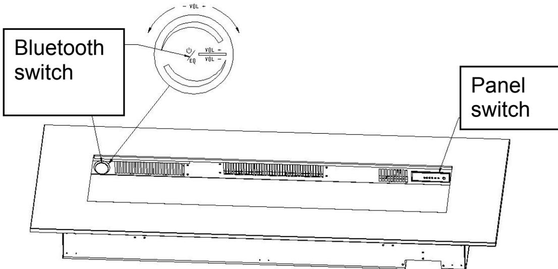
3.1 Long press the speaker boot and connect the speaker with a Bluetooth device
