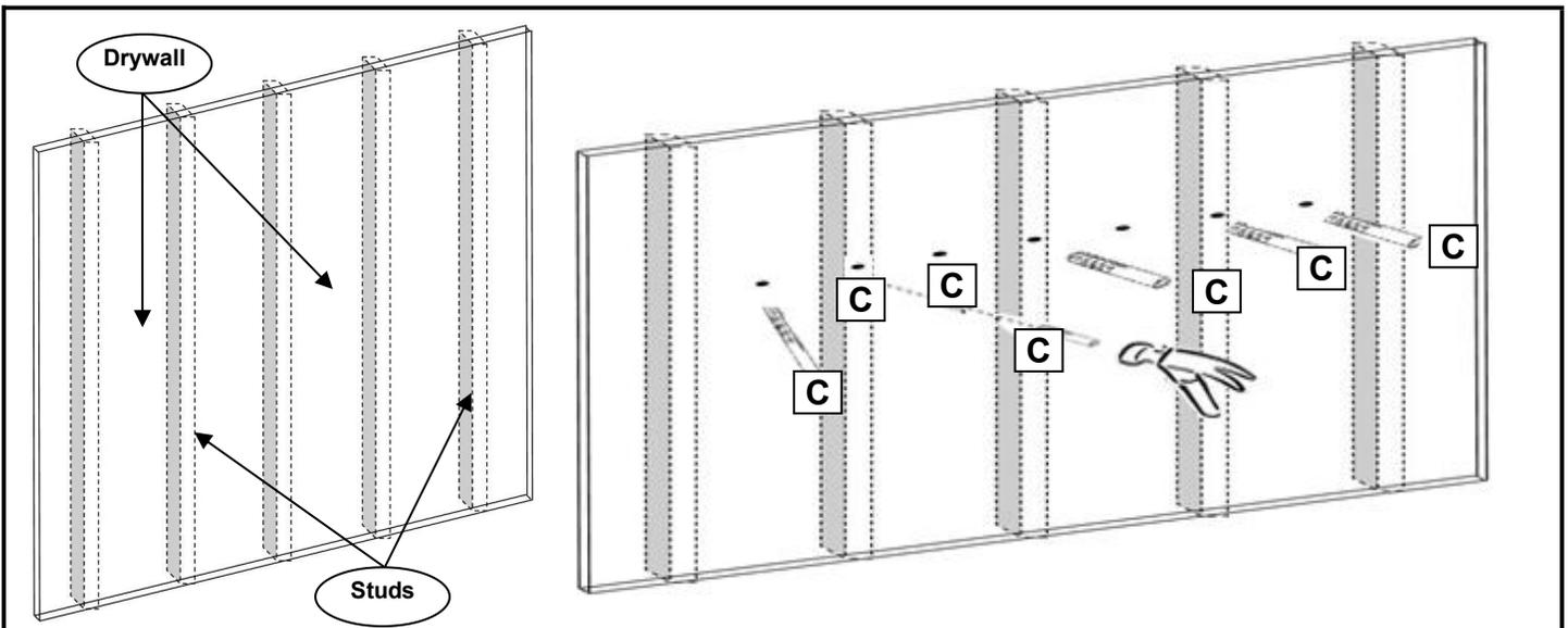
**STEP 2. A.** Locate the wall studs using an electronic stud-finder. Mark the hole locations with a pencil. The holes should be 8" (20.3 cm) apart, and level. The minimum height from the surface below must be 6" (30 cm). **B.** Three screws should be screwed directly into wall studs. Then, four drywall anchors are needed.
